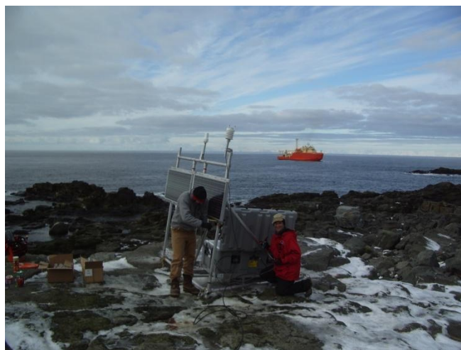
Santa Claus Rock installation off Hugo Island. Metal frame with solar panels, battery, transmission case and weather monitor with Mason Fried (left) and Eugene Domack (right) and the Lawrence M. Gould in the background. Photo by Bjorn Johns from UNAVCO.
