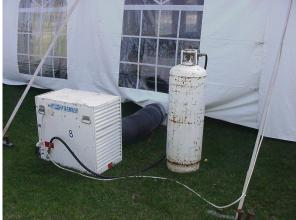
The heating device on the left is typically placed inside a tent/canopy area, where the radiant heat warms the space. As per the OFPC, this type of heating device is outright illegal in NYS, let alone in tents/canopies. So do not order these types of heating devices, and do not authorize their use in any college sponsored event.
