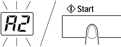
**3** While the pause function is enabled, it is possible to exit the Cycle Print Mode by pressing the Clear key a second time (the value displayed in the “No. of Copies” display will change to a “1”.)
