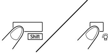
The screen is gradually darkened until it is turned OFF. When any key is pressed, the illumination returns to the maximum level.
