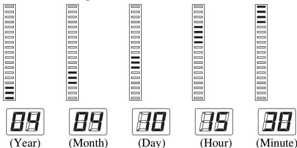
**3** In each setting mode, press the Multi-Print key to enter the setting value. Each press of the Multi-Print key increases the setting value.
